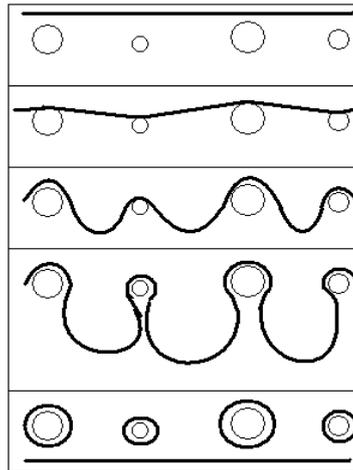
Fig. 2: The presence of foreign elements in a coating can result in a number of different behaviors of the dislocation, depending on the micro-alloying element and on the Orowan mechanism present in the matrix..
