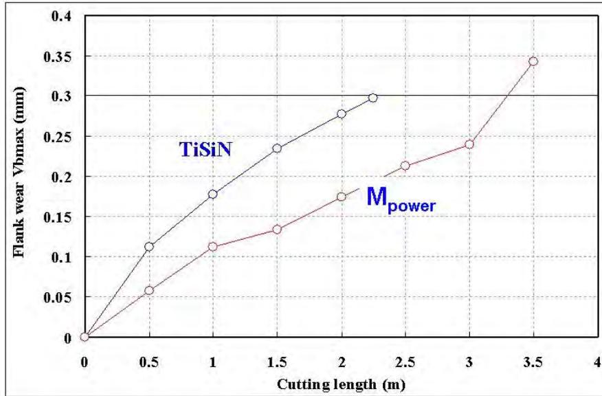
Fig. 4: M<sub>power</sub> compared to a state-of-the art TiSiN coating showing better performance in dry cutting an annealed X210Cr12 (rough milling: v<sub>c</sub>=150m/min, f<sub>z</sub>=0,15mm/tooth, a<sub>p</sub>=3mm, a<sub>e</sub>=10mm)
