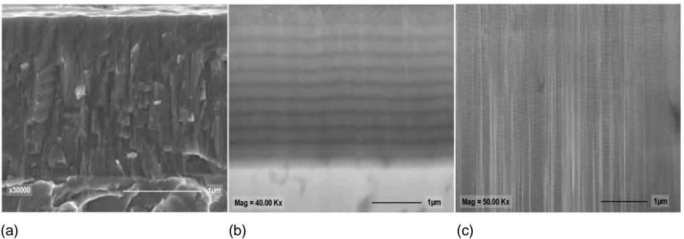
Fig. 5: The M<sub>power</sub> comes in three different coating designs, depending in the application, (a) a graded layered TiAlN and micro-alloyed MeSiXN, (b) a multilayered and (c) a nano-layered coating design
