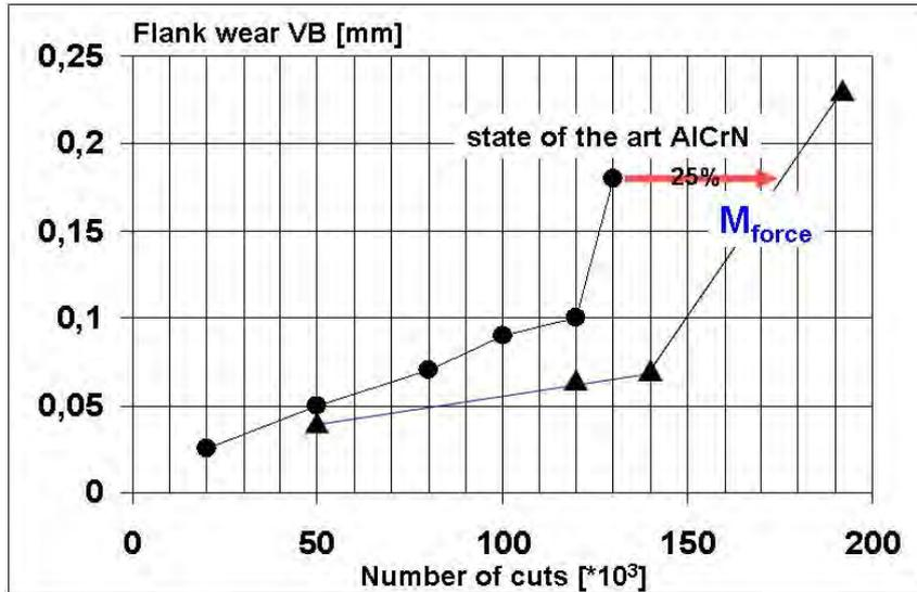
Fig. 6:  $M_{force}$  results in 25% better performance than state of the art AlCrN in dry milling on 42CrMo4 ( $v_c=200\text{m/min}$ ,  $f_z=0,12\text{mm/tooth}$ ,  $a_p=3\text{mm}$ ,  $a_e=3\text{mm}$ )
