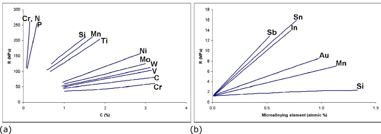
Fig. 1: (a) Microalloying of steel: the effect of microalloying on the yield strength  $R$  of steels depends on the nature and the amount of the microalloying element. (b) The effect of the nature and the quantity of the microalloying elements on Cu yield strength ( $R$ )
